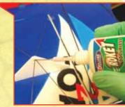
Front and rear fuselage halves are glued to the wing using Foam 2 Foam glue giving a strong, flexible joint.
