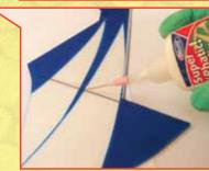
6 Carbon aileron supports are glued in place, adding rigidity whilst keeping weight to a minimum. The needle applicator used with the Roket Odourless cyano controls the glue application.
