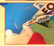
Servos are bonded in to the fuselage using small dots of Roket Odourless cyano.
